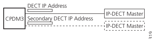
Figure 25. Communication with the IP-DECT system is done over a LAN
